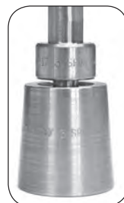
Male sits higher on base. This gap prevents teeth on spur grommets from getting crushed when set.
