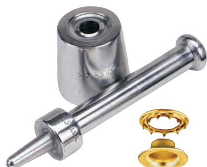
Male sits higher on base. This gap prevents teeth on spur grommets from getting crushed when set.
